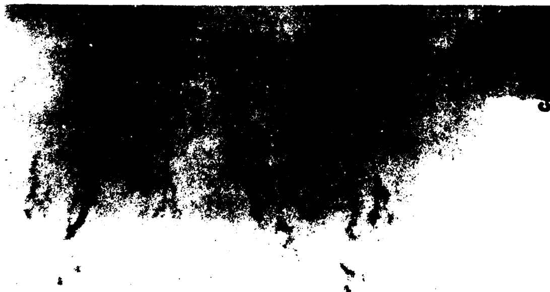
FIG. 3 - Illustration of Shrinkage, Type 1, Category C, Severity level 5 - from ASTM E-186, Reference Radiographs for Steel Castings.
