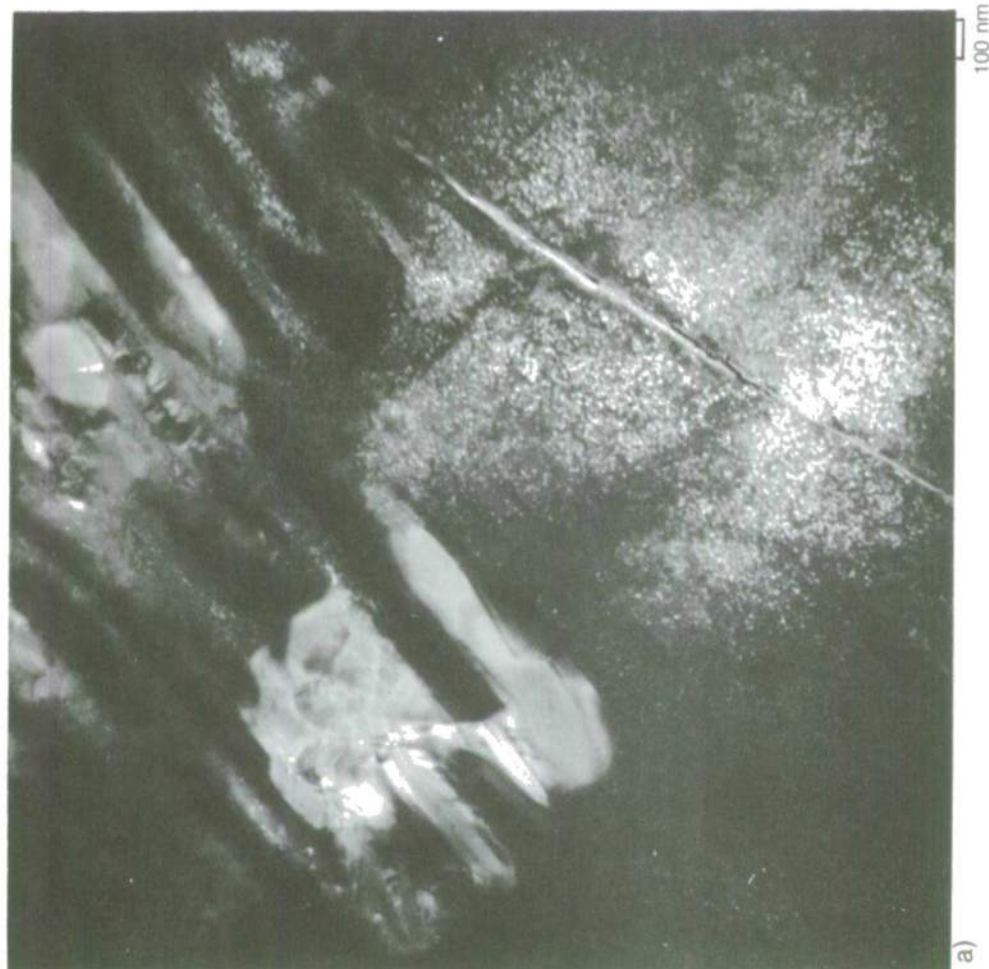
a) DARK FIELD PHOTOMICROGRAPH OF FINE \text{Ni}_4\text{Mo} PRECIPITATES IN \gamma NEAR CELLULAR POCKET, g = 110 \text{ Ni}_4\text{Mo}
