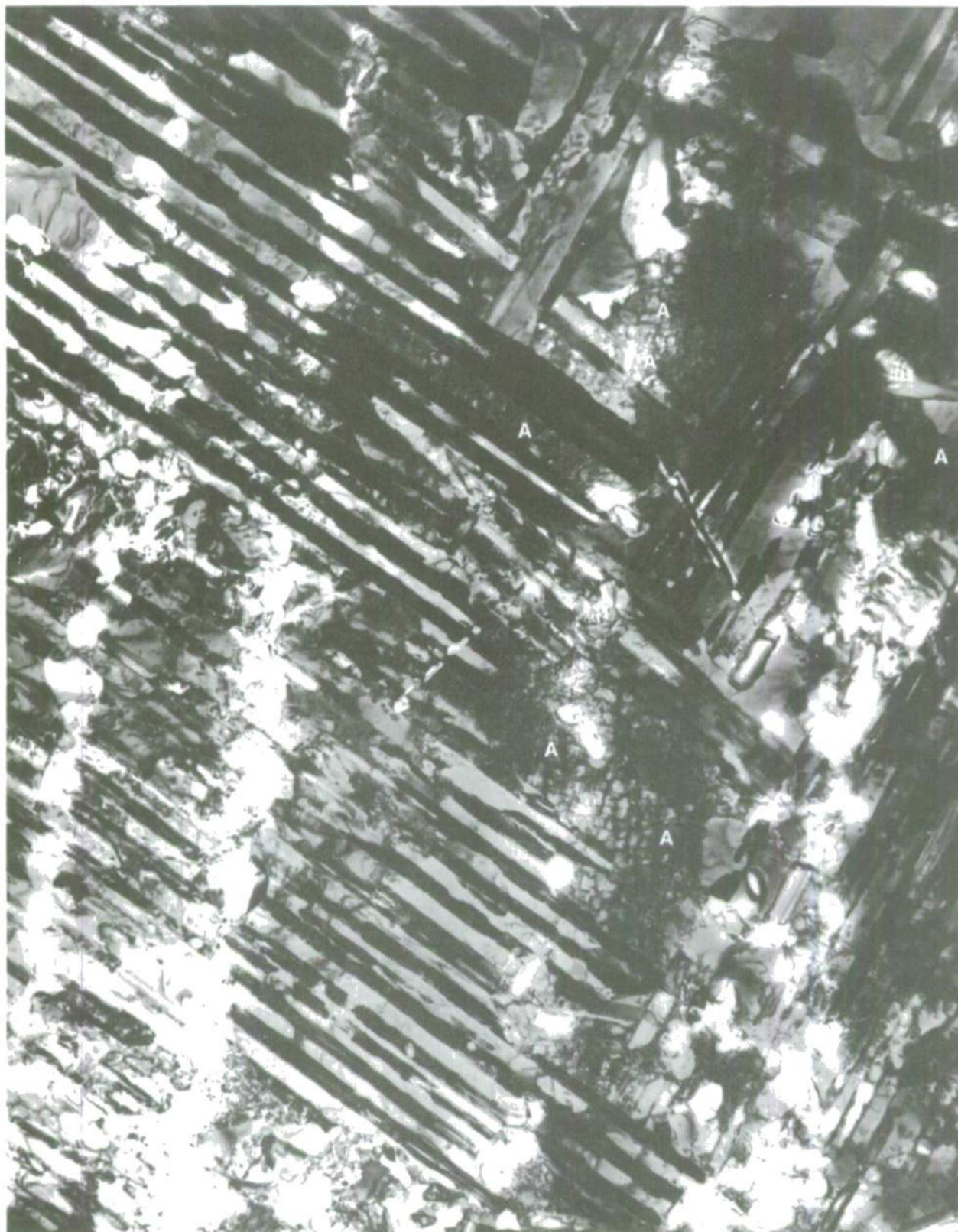
LAMELLAR STRUCTURE IS ORTHORHOMBIC \text{Ni}_3\text{Mo} AND \gamma' UNTRANSFORMED AREAS OF \gamma + \text{Ni}_3\text{Mo} AND CUBOIDAL \gamma' ARE VISIBLE IN SOME AREAS (A)
