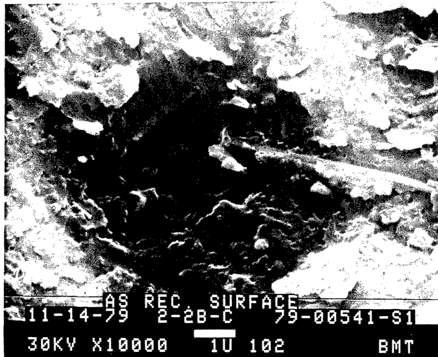
Figure 46. Failure Surface of PL-728/PL-729-3 on 2024-T3-Bare FPL
