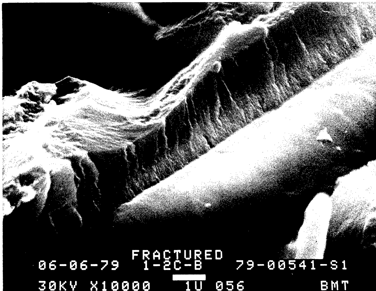
Figure 32. Transverse View of Failed Specimen—2024-T3-Clad, PAA Oxide, BR-227 Primer, FM-61 Adhesive
