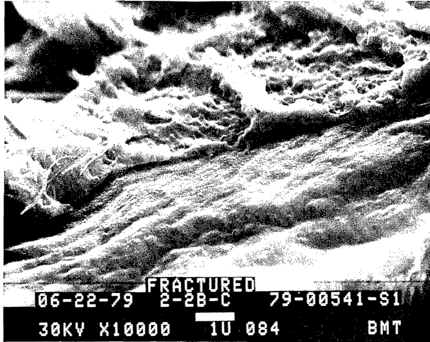
Figure 42. Transverse View of PL-728/PL-729-3 Failure Surface on 2024-T3-Bare FPL
