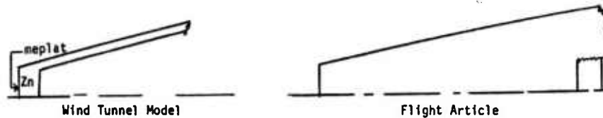
Schematic of Difference of Tip Configuration Between Wind Tunnel and Flight Article
