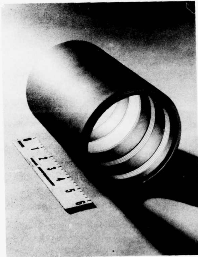
Figure 19 Metalized beryllia insulator for 673H collector.
