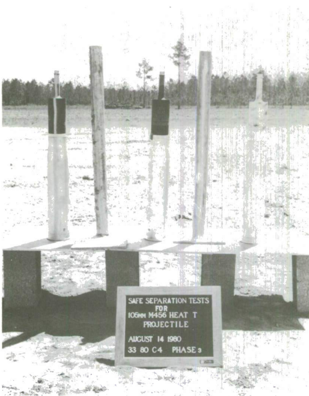
Figure 15. M456 Cartridge, vertical - shielded, pre-test view
