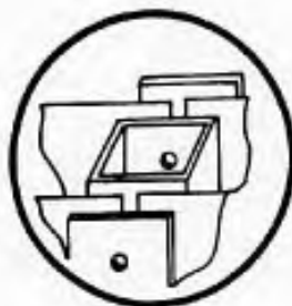
Figure 5. Typical seam-joining hardware for true cell-type room.
