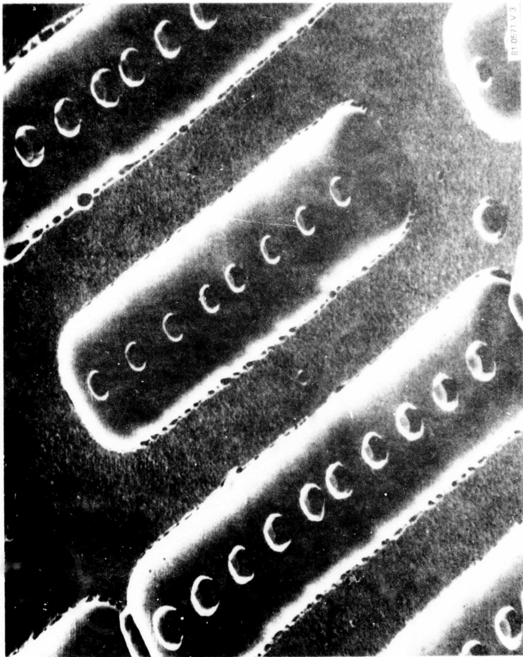
Figure B-6. Scanning Electron Micrograph of Etched Tub and Vias
