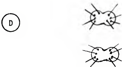
Figure 3.3-3. An Illustration of a non ionic Emulsion and how Tramp Oil will React with it.
