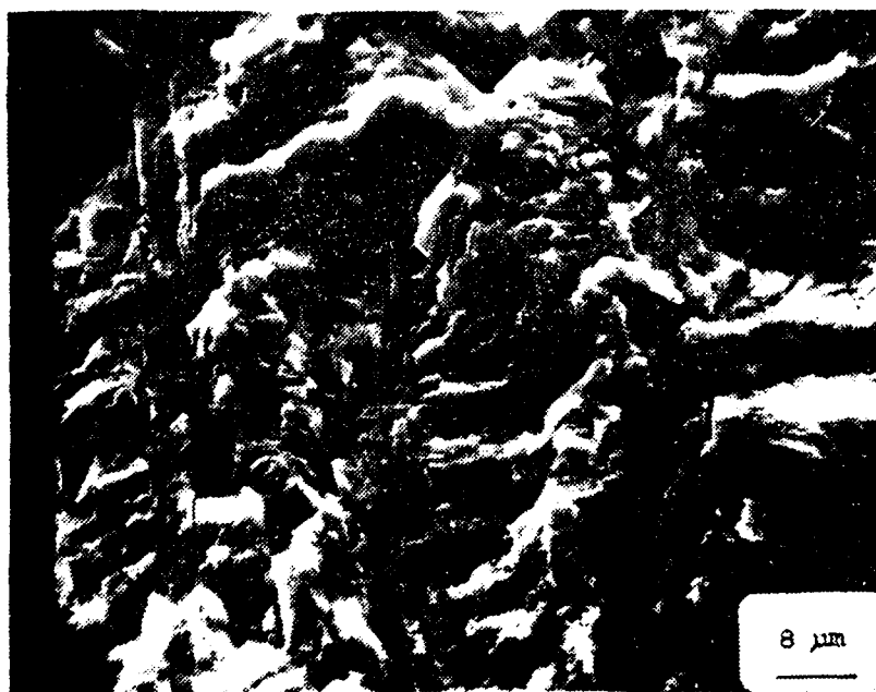
FIGURE 30. (a) Fully developed Stage II crack growth on same specimen shown in Figure 29; magnification 1100x SEM; (b) Stage III fracture appearance; magnification 1250x SEM
