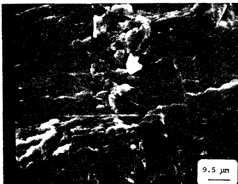
FIGURE 27. (a) Regions of Stage II crack growth in a specimen of Al-10.2 wt pct Mg oil-quenched from homogenization temperature which fractured after 1.81 \times 10^5 cycles: (b) overload region of the same specimen (SEM x 1050)
