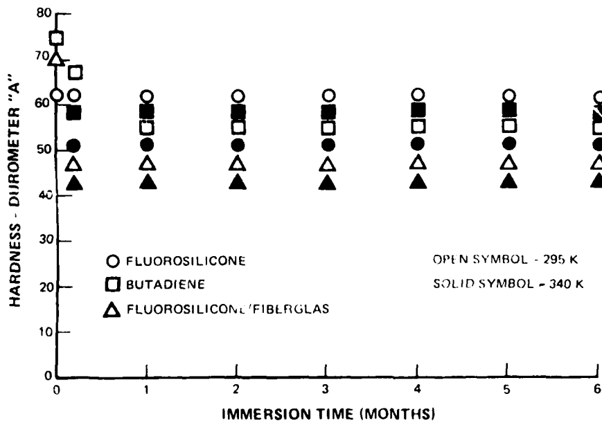
Figure 43 Effect of Hardness On Elastomers Immersed In AMK
