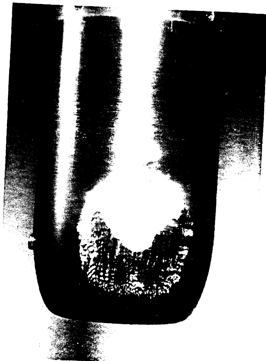
Figure 37. Photograph of two types of transient cavitation on the DTNSRDC nose. The large cavity is a travelling patch. At top is a travelling bubble. ( U_{\infty} = 50.0 fps, \sigma = 0.525 , \alpha = 9.0 ppm)
