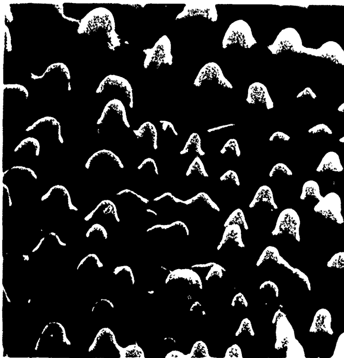
Figure 40. A-77-205 \gamma - \gamma' - \alpha (Ni Mo Ta Al) after testing showing area of arcing. x 10K C4847
