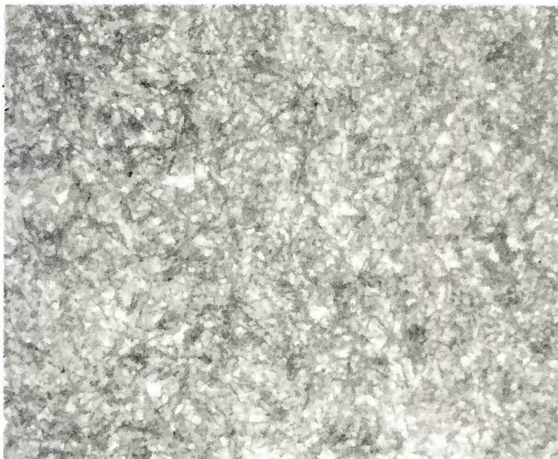
Figure 25. Photomicrograph of untempered martensite with very little amounts of retained austenite. This sample was austenitized at 815°C (1500°F). 1000x
