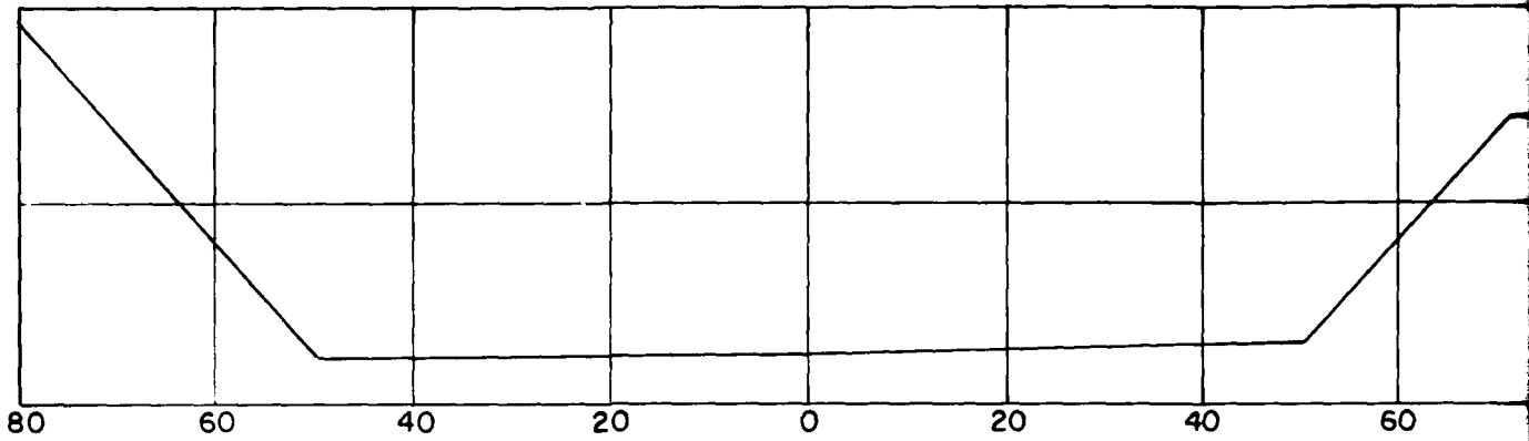
SPILLWAY SECTION 25 FT. LEFT \& DAM
