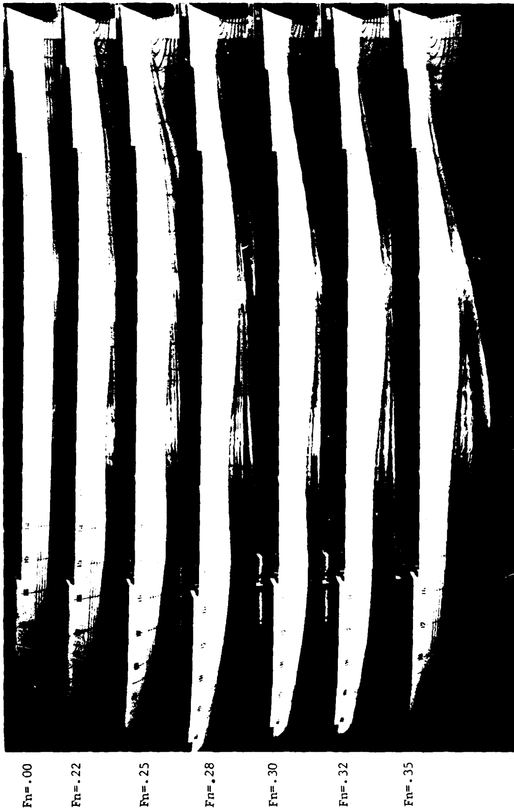
Figure 3 - Wave Profiles for Model Free to Trim and Sink
