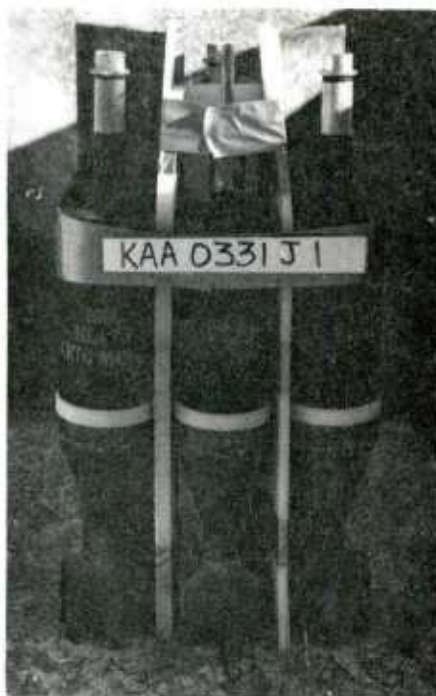
DONOR AND ACCEPTOR PROJECTILES BEFORE TEST
