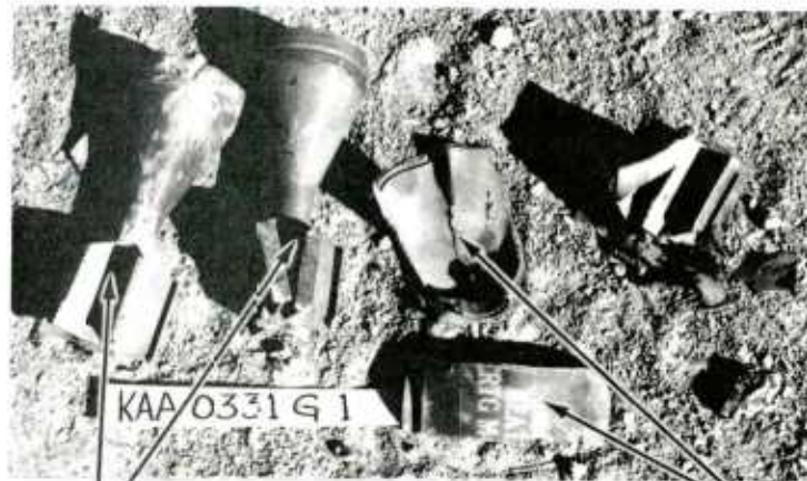
FRAGMENTS OF ACCEPTOR PROJECTILES RECOVERED AFTER TEST
