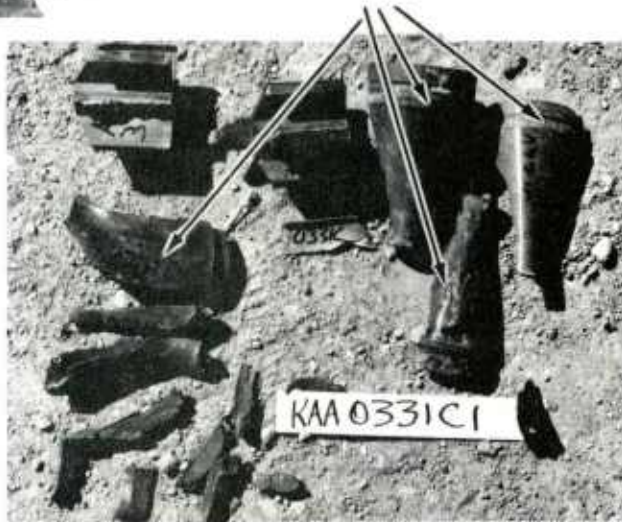
FRAGMENTS OF ACCEPTOR PROJECTILES RECOVERED AFTER TEST
