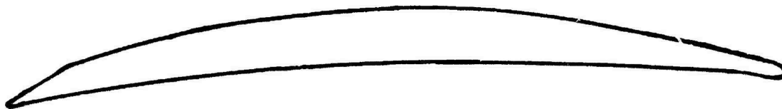
REFURBISHED FAN PROFILE WITH CHISEL CUT
