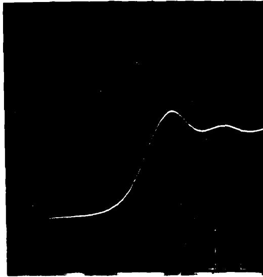
Figure 16. Output Step Function ( V_o ) from Line Pair No. 5, Figure 8, with Coupled Line Terminated with 50 ohms. ( s = 10 mils, W = 5 mils, l = 2.54 cm). Vertical = 50 mV/div.; Horizontal = 50 ps/div.
