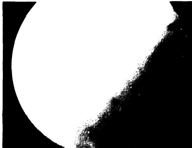
Figure 95. Nomarski 2 interference contrast micrograph of sample L16, 1.2 \text{ J/cm}^2 double-frequency laser-irradiated.
