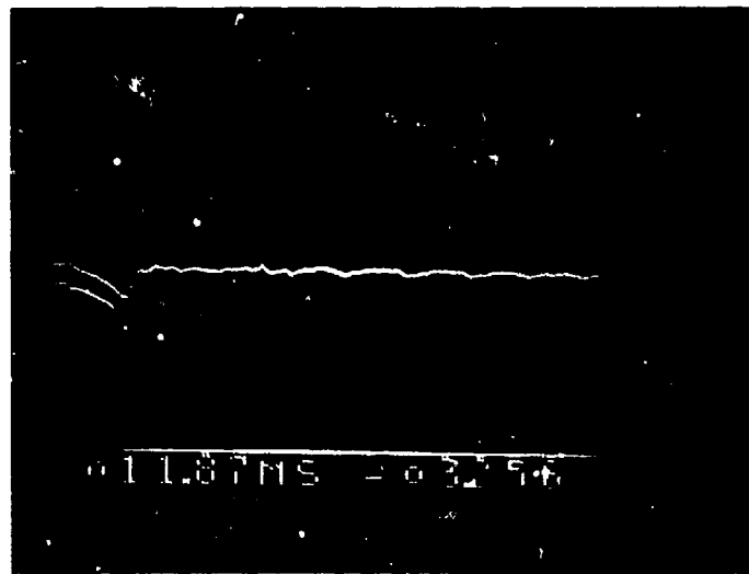
FIGURE 3.5a: THE UPPER AND LOWER TRACES CORRESPOND TO THE RESPONSE OF STRAIN GAGES A AND B, RESPECTIVELY. (SPECIMEN KE2)
