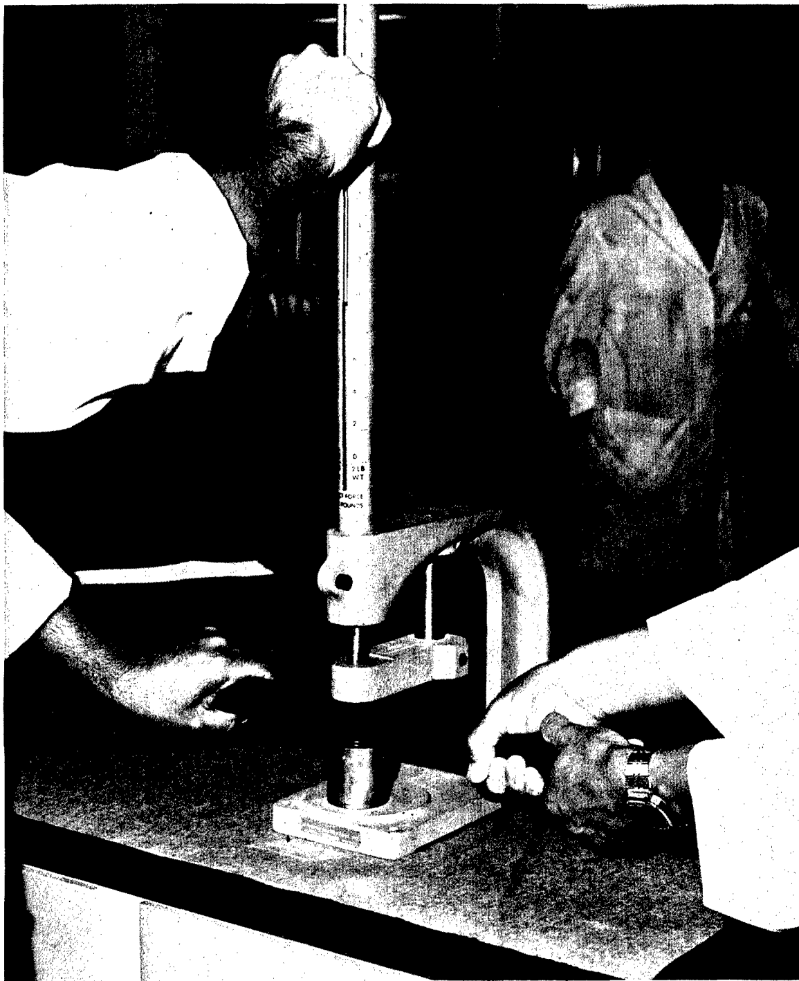
Figure 2. Method Used to Impact Damage the Coatings on Test Panels and Torsion Bars
