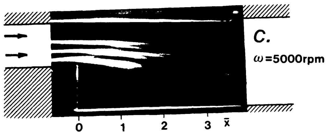
Figure 78. Streamline Shapes for Various Rotor Speeds, \bar{h} = 1.
