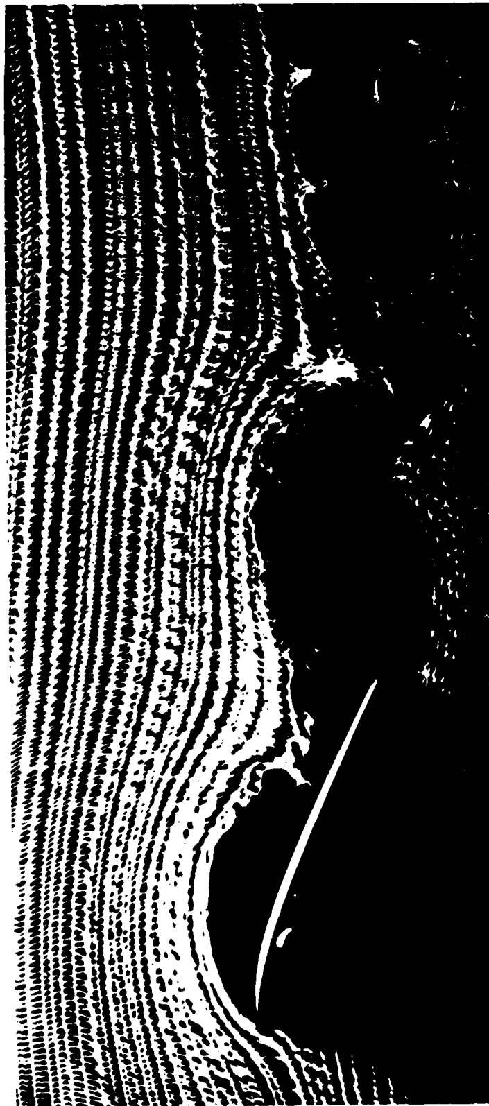
Figure 49. Hydrogen Bubble Flow Visualization of the Field Around an Oscillating Airfoil (from McAllister and Carr, Ref. 37A)
