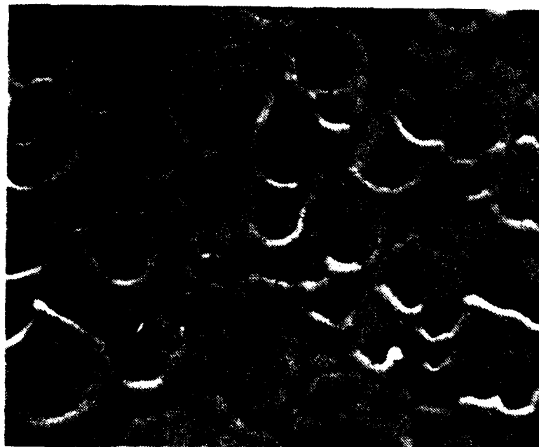
Figure 53. 1030 Steel. Unipolar arcs found at 2.0mm distance from main laser crater (1250X SEM)
