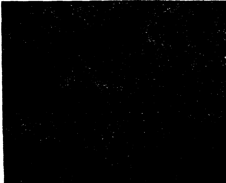
Figure 47. Copper. Scintillation pattern produced by x-rays from silica coating on copper surface seen in previous figure (1200X SEM)
