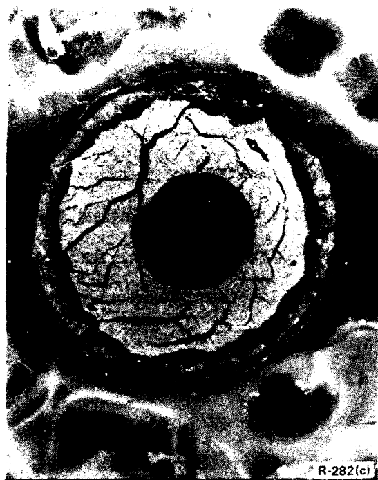
Fig. 41 — A cross section through a tubular plate. The tube can be seen as a thin dark line around the edge. The dark area within the tube, with the very irregular inner boundary, shows the extent of the sulfuric acid penetration after one minute of soak. The lighter zone within this circle is untouched powder. The dark circle at the center is the spline that extends through the tube as a current collector. The tube was impregnated with plastic before sectioning, and the apparently open cracks are actually filled with the plastic. Magnification 8X.
