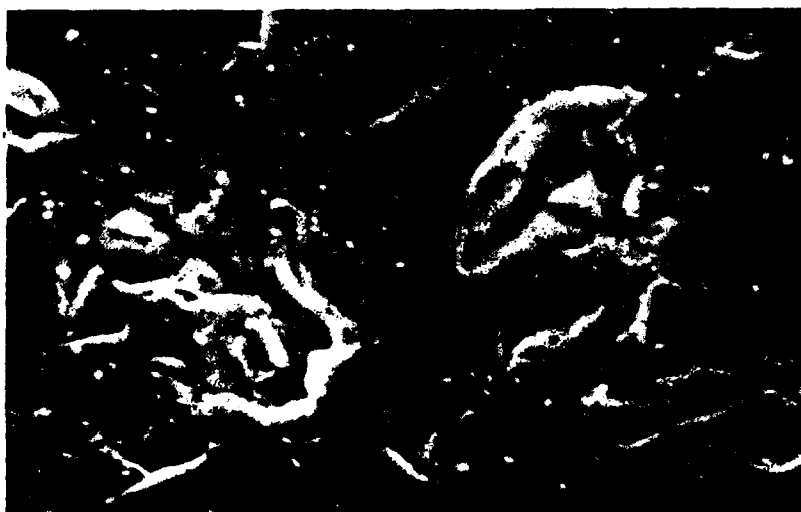
Figure 12. SEM Micrographs of Single Impact Craters of a Copper Target
