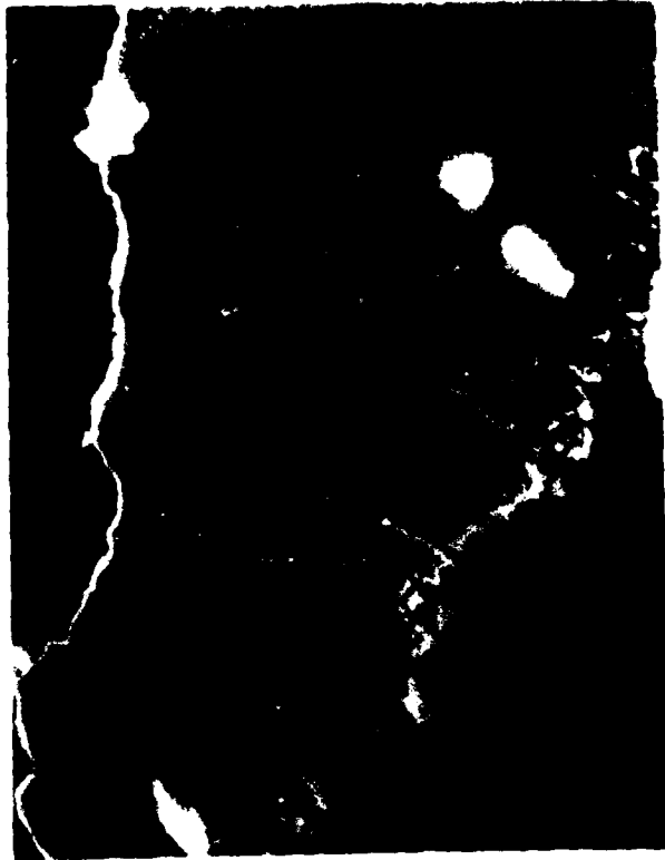
7. SEM micrograph of large wear fragment presumed to be a broken out extrusion (7.5 Al-Cu alloy lubricated with 1% stearic acid in octadecane). (540x)
