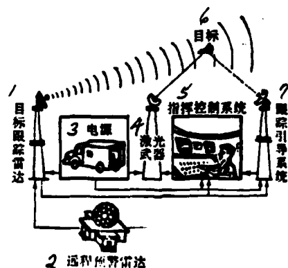
Fig. 9-5. The main constituents of a laser weapon.
