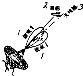
Fig. 7-12. Principle of signal comparison. Key: (1) Beam; (2) Target; (3) Axis of antenna.
