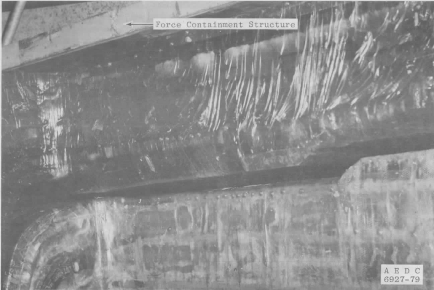
Figure 36. Nonuniform spacing between coils no. 2 and no. 4.
