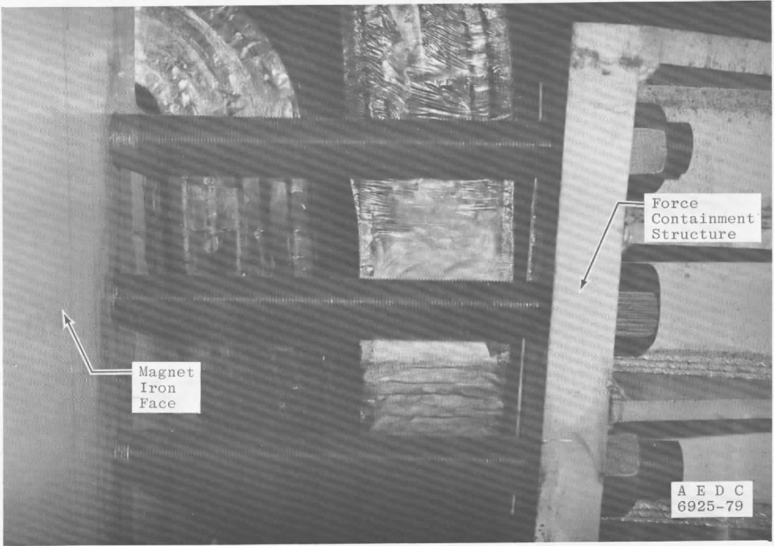
Figure 33. Nonuniform spacing on coils no. 2 and no. 4.
