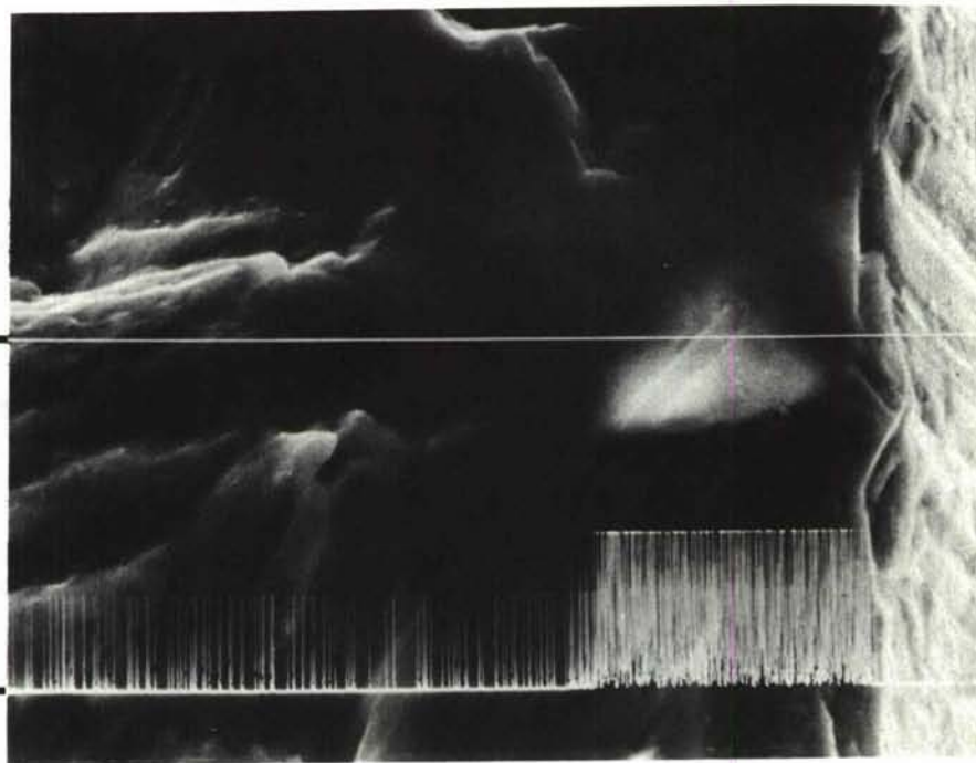
Fig. 22d CT91 forging (L), 1624 N_f initiation site D.
