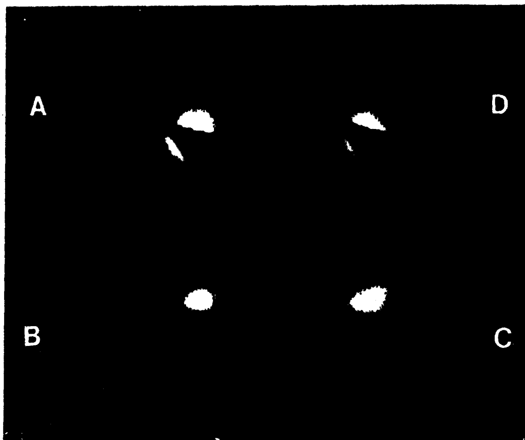
Figure 23. (a) Original, diffraction-limited image (b) Aberrated image (c) Aberrated and defocused image (d) Resulting image after (b) and (c) are used to form a point estimate of the phase aberration and the blurring.
