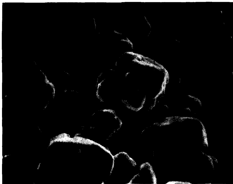
Figure 78. Micrograph of Sylvania Tungsten Powder After Sorting and Deconglomeration 5.5-6.5 \mu\text{m} Nominal Size.
