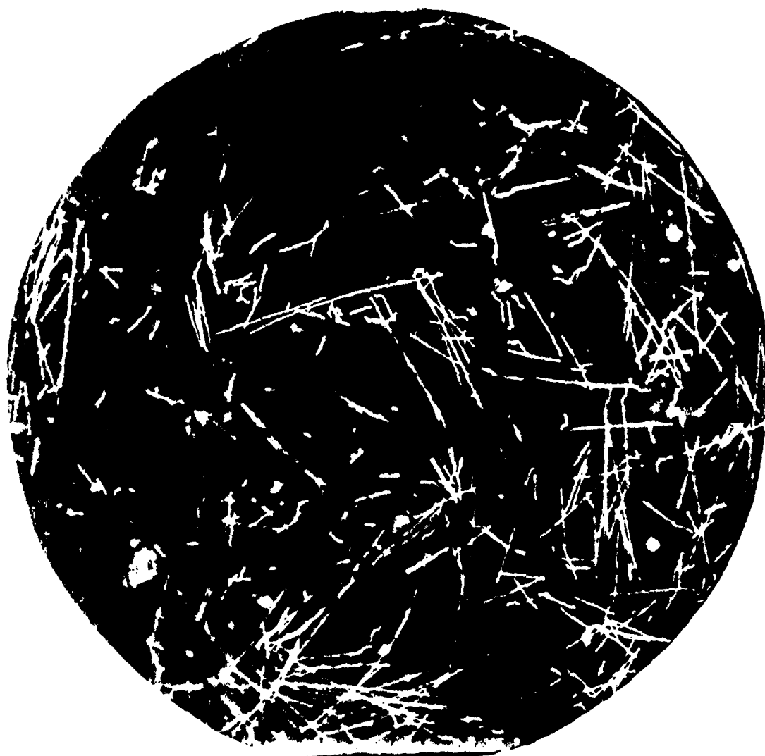
Fig. 2.11. X-Ray View of a Typical 1/2 Inch Slice of a 6 x 12 inch Cylinder Vibrated Internally.
