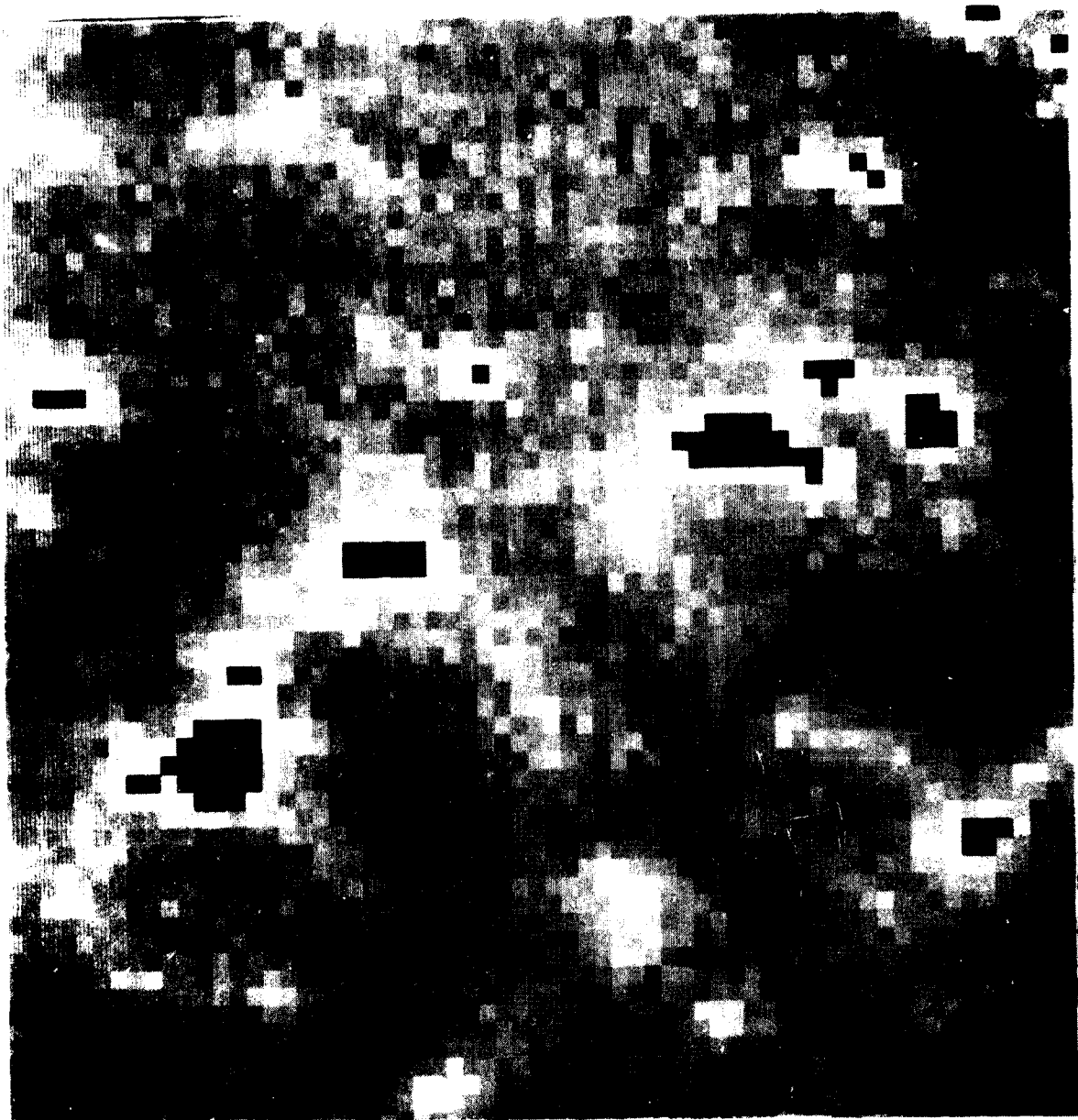
Figure A-5 Magnified digitized image of blotched whitecaps with minimum brightness set at 160
