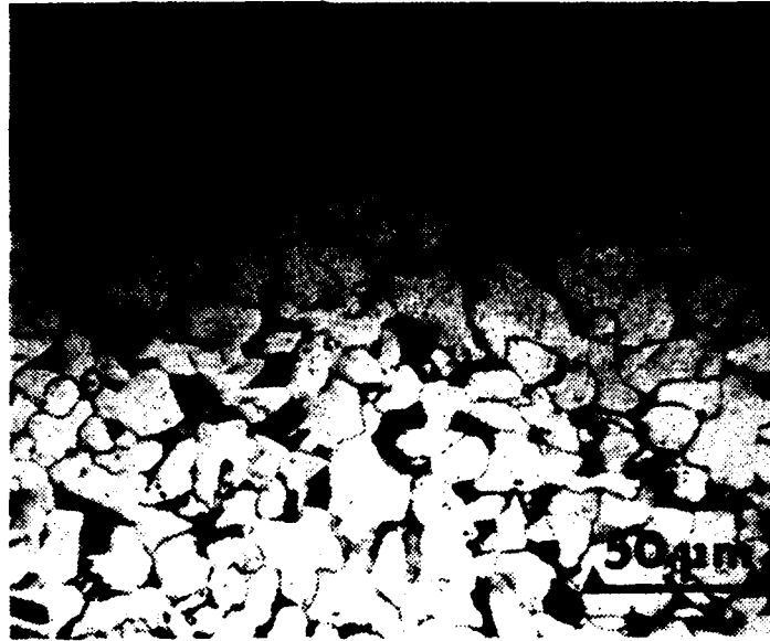
Figure E-2. Optical Micrograph of Ferrite-Pearlite Structure of 1020 Steel. Magnification 400X.
