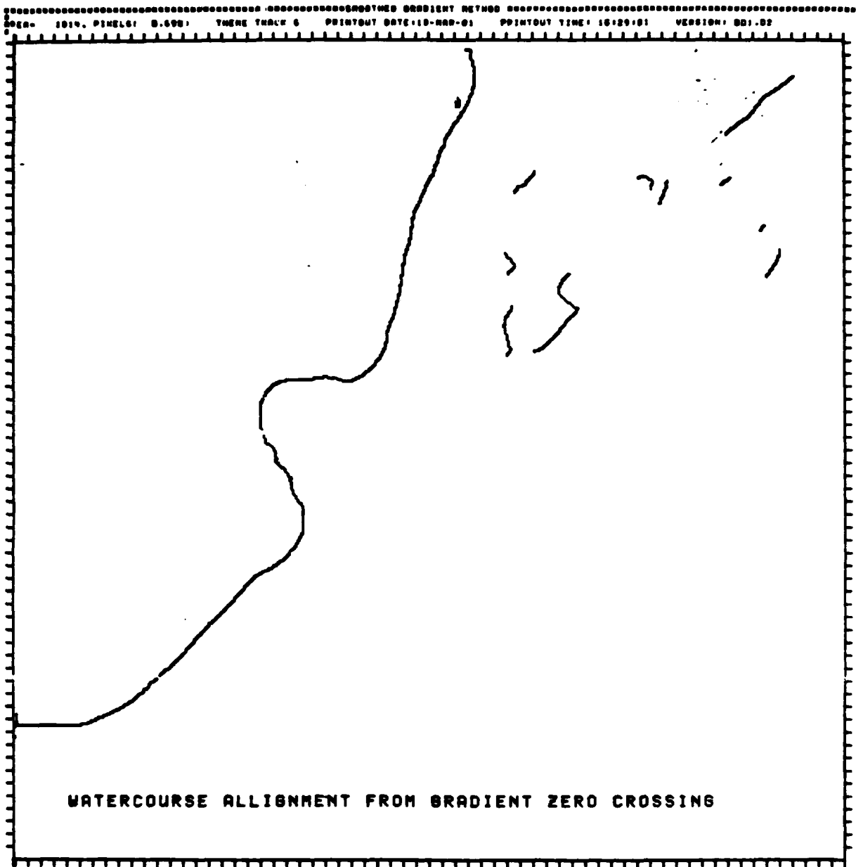
Figure 8. Watercourse Skeletonizing by Gradient On Spatially Simple Stream
