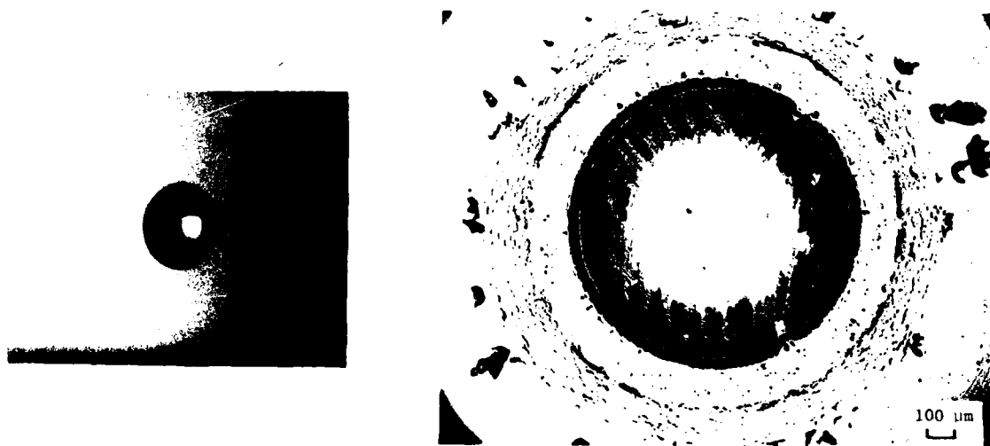
b. Distorted Water Drop Impacting at 495 \text{ ms}^{-1} (Aspect Ratio 1.19).
