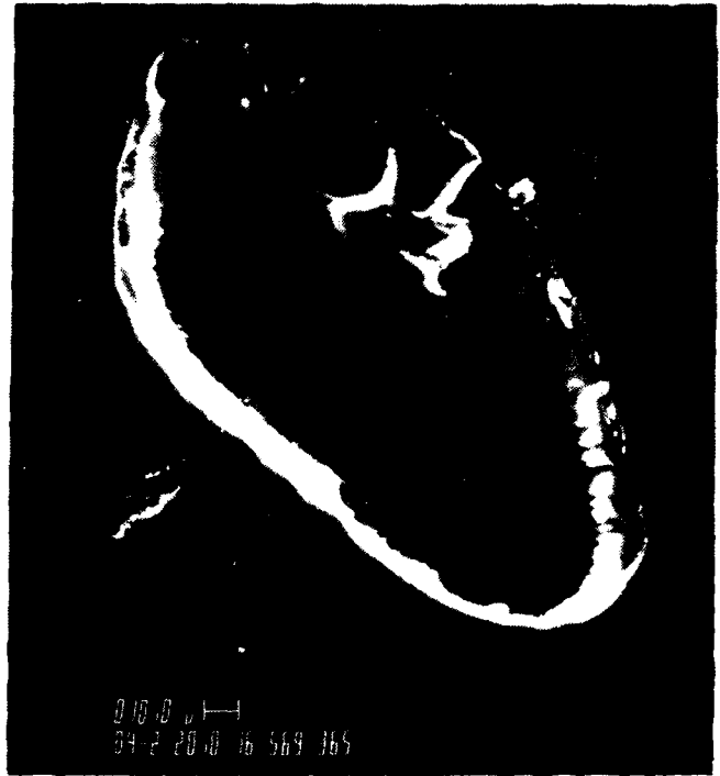
B 1.0 min Rain Exposure
