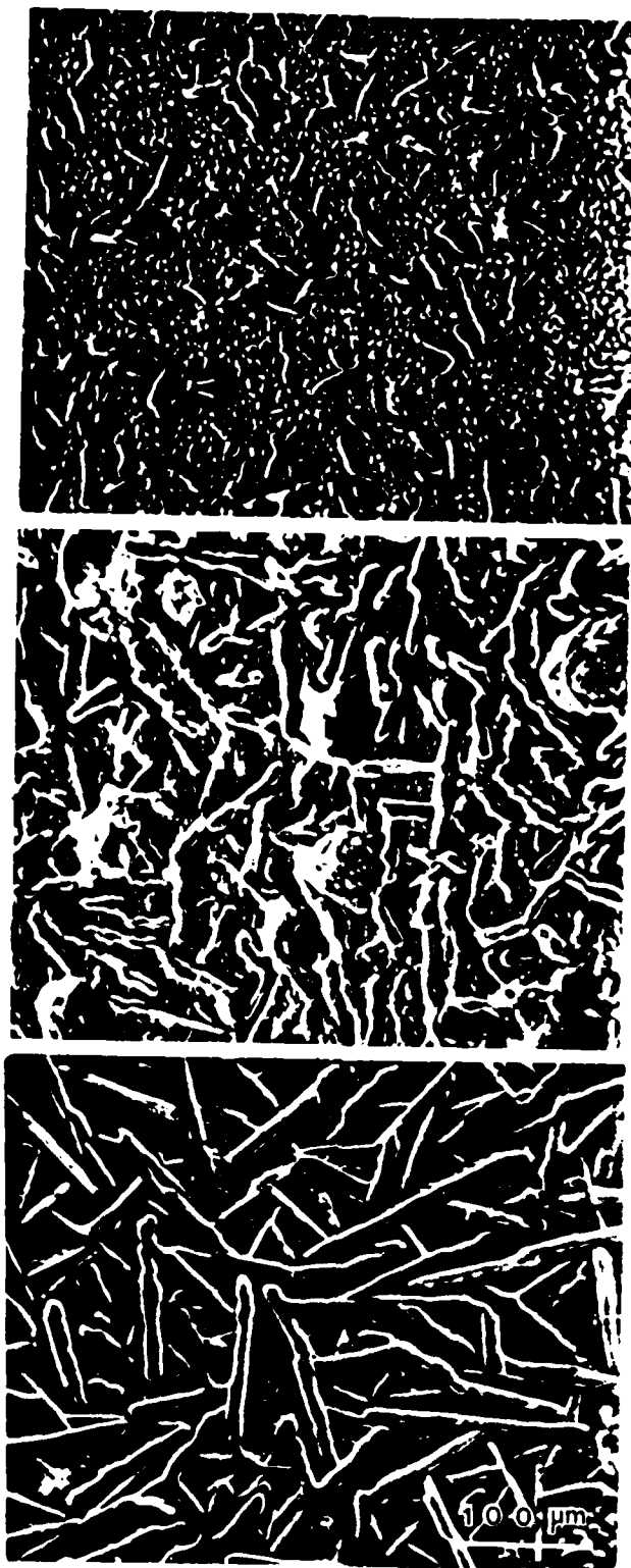
Fig. 1. SEM micrographs of \text{Si}_3\text{N}_4\text{-8\%Y}_2\text{O}_3 oxidized at 1450^\circ\text{C} for (a) 80 min, (b) 48 hr and (c) 2 hr.
