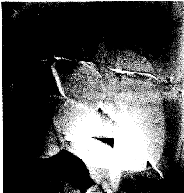
Figure 4 SEM photomicrograph of sample SN502-95-13 which was fired at 2145^{\circ}\text{C} under 2.2 MPa of \text{N}_2 for 60 minutes. (10,000 X).
