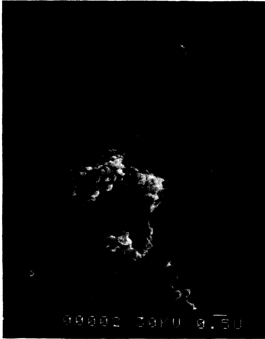
Figure 31. SEM Photograph of Engine Exhaust Particulate Sample Collected During Tests with JP-4 only on 10 November 1981 (10Kx Magnification)
