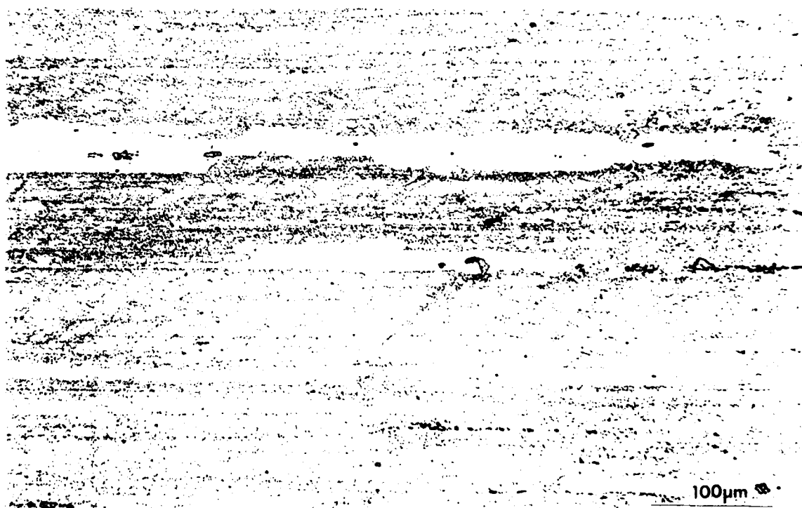
FIGURE 17. LONGITUDINAL MICROSTRUCTURE OF 7475-T7351
