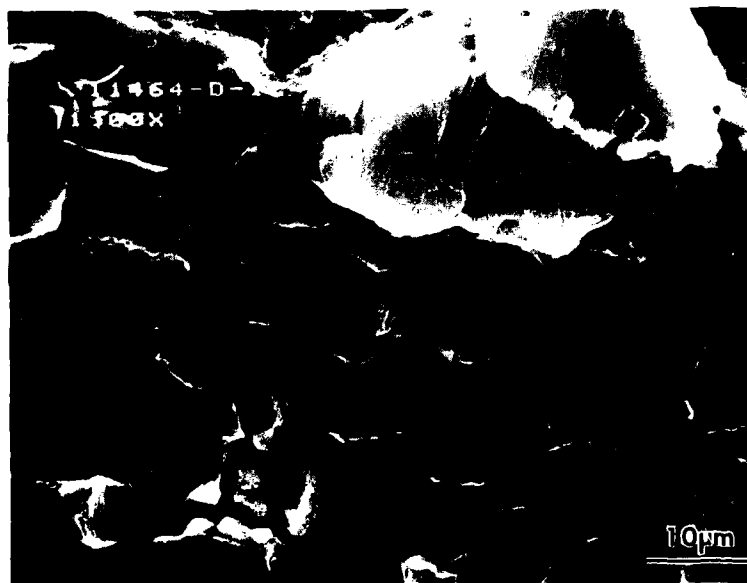
FIGURE 37. FRACTURE SURFACE OF 7050-T73651 AT a = 6.4\text{MM} (0.25 IN.) TESTED UNDER TD SPECTRUM
