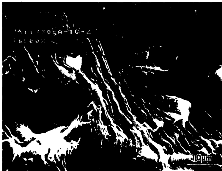
FIGURE 34. FRACTURE SURFACE OF 2024-T351 TESTED USING TD SPECTRUM
