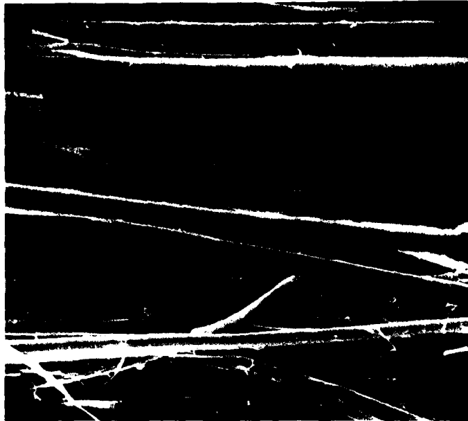
FIGURE 2. TRANSVERSE FRACTURE APPEARANCE OF KEVLAR 49/934 COMPOSITE IN DRY CONDITION. 450X.
