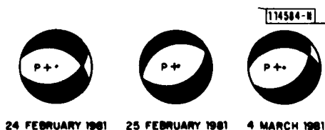
Fig. III-12. Fault-plane solutions (major double-couple) of three closely spaced earthquakes in Southern Greece.
