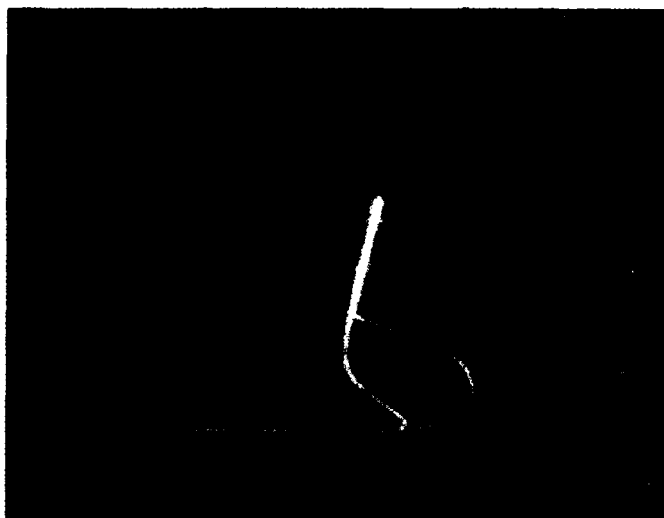
Figure 8. I-V characteristic in CD4061A, S7 between V_{DD} and V_{SS}
