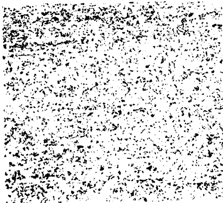
B. Gleeble simulation ESW 1000 kJ/inch.
