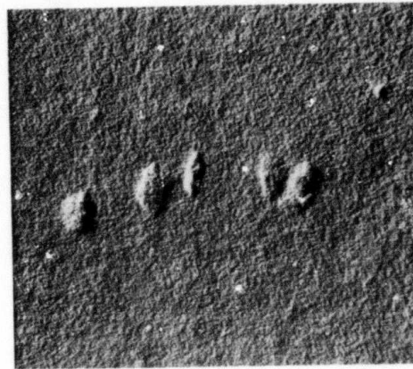
(B) CARBON INCLUSIONS - BOTH COMPUTERIZED OUTPUTS ARE OF 0.010 INCH CARBON.
