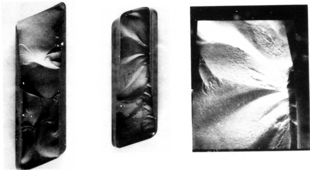
Figure 6-15. SEM Photomicrographs Showing the Fractured Surfaces of Blades that Fractured Below the Platform in Test 17 of Engine CE001.
