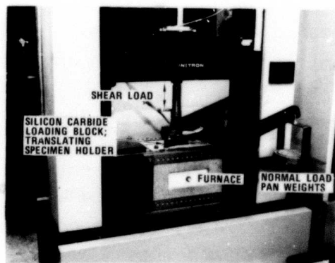
Figure 7-2. Schematic and Photographs of the Contact Test Apparatus.
