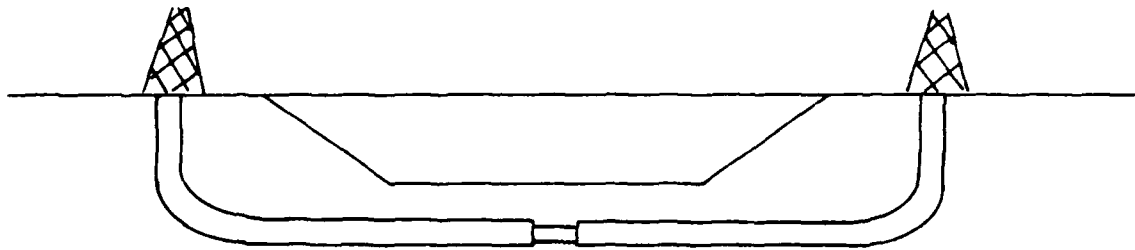
Figure 2a. Bottom Sealing of a Lagoon via Directional Drilling
