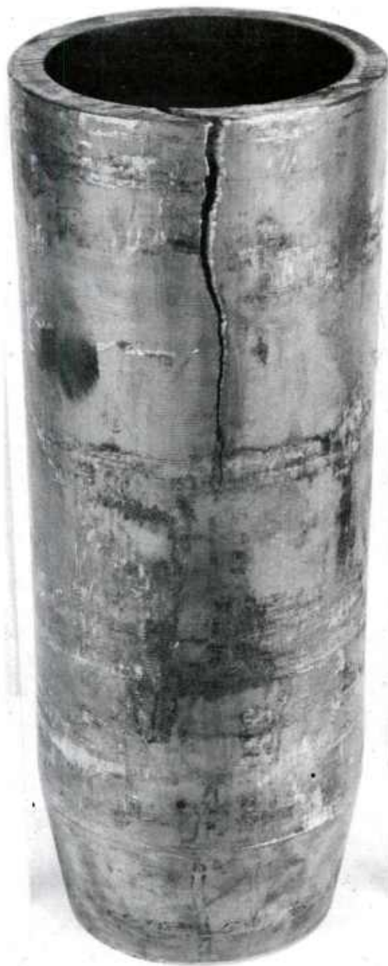
Figure 27. Defective forging made from Roblin Steel product
