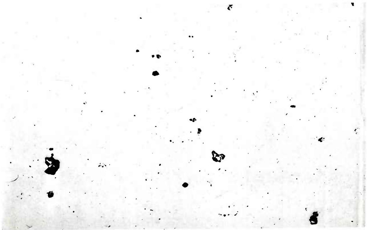
Figure 2. Microporosity at center of bar section 1A - Republic Steel (100X)
