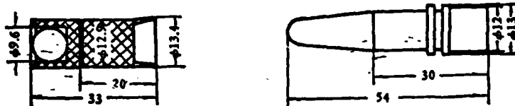
Figure 7. Schematic diagrams of the spherical model and its evolution body launched by a light gas gun.
